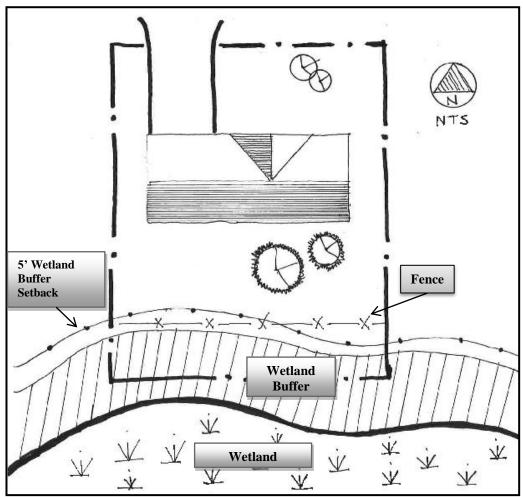
Example of a single-family residential lot with wetland buffers on the property. As shown on the sketch, the wetland feature is offsite, but the wetland buffer extends onto the subject property where improvements are generally not permitted. A five-foot building setback from the wetland buffer is also shown. Only limited improvements, such as fencing, are allowed within ECA buffer setbacks.
